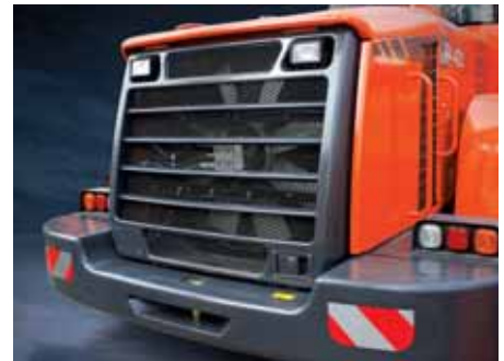
Radiator Grill (Steel structure)
